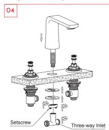
Place the faucet body downward through the basin deck. Then put on the rubber washer and locking washer, tightened by diamond-shaped nut and setscrew. Connect the three-way inlet.
