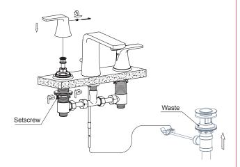
Loosen the M5 screw first. Take off from the inlet valve bodies the following one by one: handle, locking washer, plastic spacer and decorating ring. Screw off the locking nuts to the bottom.
