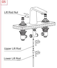
First connect the upper lift rod with the lower lift rod. Then insert the lift rod nut into the slot at the back of the faucet body to connect with the upper lift rod.
