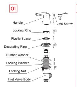
Loosen the M5 screw first. Take off from the inlet valve bodies the following one by one: handle, locking washer, plastic spacer and decorating ring. Screw off the locking nuts to the bottom.
