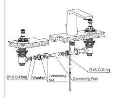
Use the connecting rod to connect the two inlet valve bodies and the three-way inlet. Tighten them with connecting nuts.
