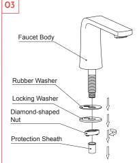
Take off the following from the faucet body accordingly: the protection sheath, diamond-shaped nut, locking washer and rubber washer.
