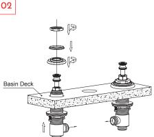
Place the two inlet valve bodies (red on the left and blue on the right) upward through the basin deck with the outlet holes facing against each other. Tighten on the deco rings. Put on the plastic spacer and then tighten the locking rings.
