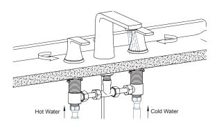
After installation, turn on water to check if everything is complete. Attention to cold water on the right and hot water on the left. The diagram shows water flow when the handles are turned on.
